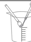
**2** Look at the bottom side of the carriage. Using the cleaning stick dampened with the maintenance cleaner, moisten the surface of the print head nozzles.
