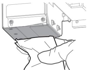
**4** If the ink cannot be removed completely, remove the emitting window glass from the lamp and use the supplied scraper to clean it off.
