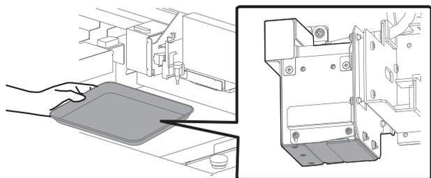
**3** Use a paper towel to clean dust or ink off the underside of the UV-LED lamp.
