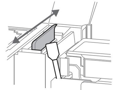
**3** Use the cleaning stick to remove the ink and dust on the circumference of the cap.
