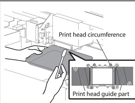
**2** Use the cleaning stick to remove the ink and dust on the bottom of the carriage.
