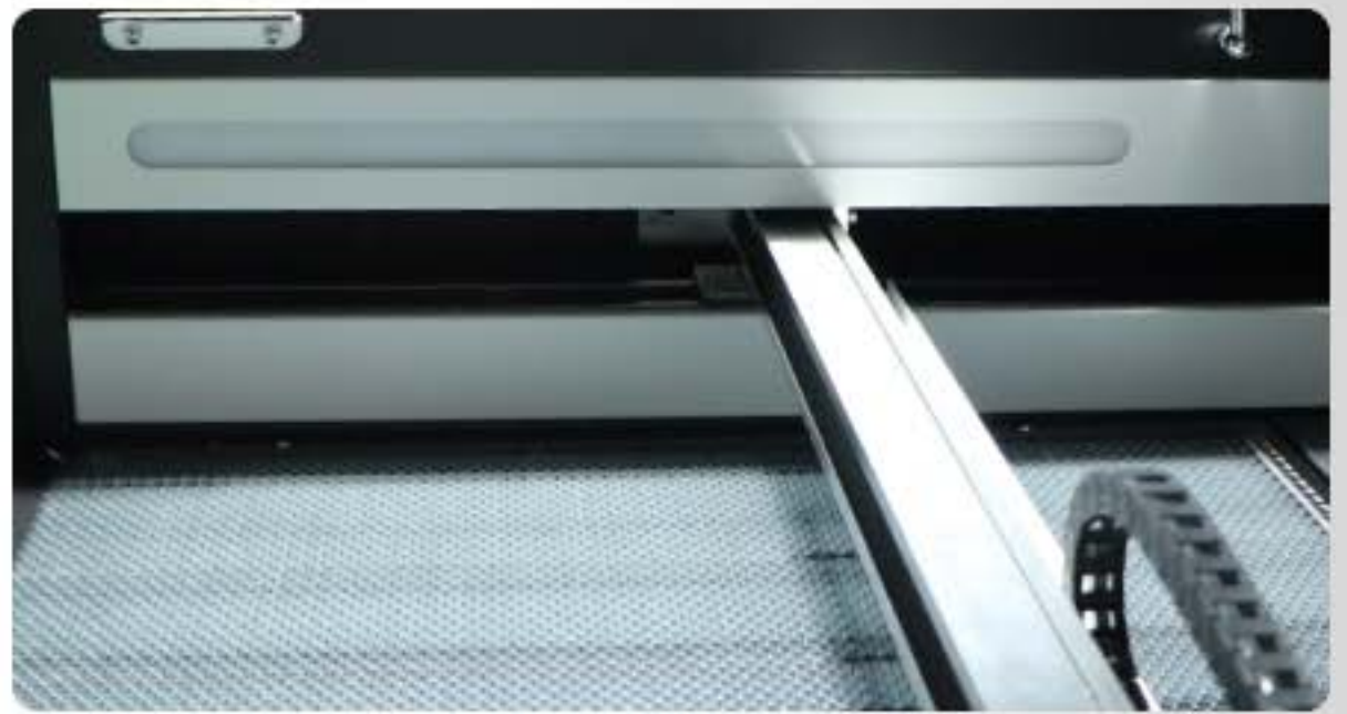
Fully enclosed dust-proof guide rail
