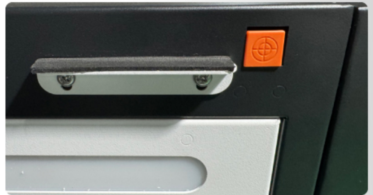
Close the cover and the laser will work normally; open the cover and the laser will stop working; which is safety
