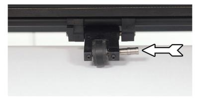
Push the pinch roller shaft in the pinch roller block while tightening the grub screws to secure the pinch roller shaft in the pinch roller block.
