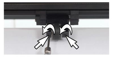
Push the shaft out of the pinch roller block from the left side towards the right side.
