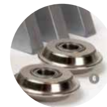
6 Scoring tool: 32 mm diameter, 1 mm round crest.
