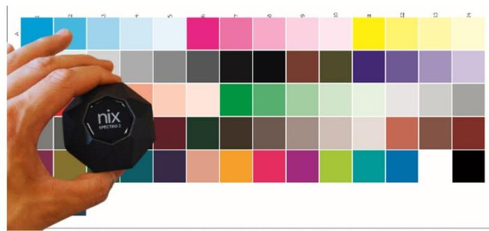
Figure 15 – NIX Spectrophotometer and the ONYX Weekly Baseline Swatch
