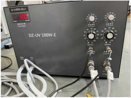
(It is recommended to mix 30-40% antifreeze with 60-70% purified water and pour it into the water tank).
