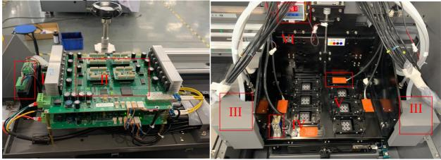
I. Z step driverII.Carriage boardIII. LED lampIV. Z height detection sensorV. Head plate heating barVI. Head plate heating controller
