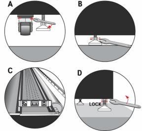
2. If hard to move by Omni-directional wheels, try move to different directions to make the wheels get same directions then easy to move
