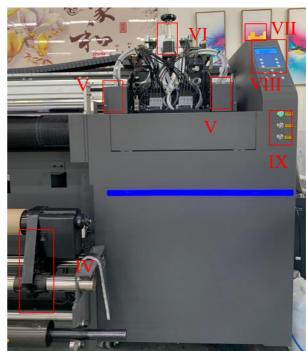
I. Table Vcuum pump II. Table vacuum area III. Media collecting control button IV. Machine collecting media parts V. LED lamp VI. Z movement step motor VII. Emergency stop button VIII. Machine control panel
